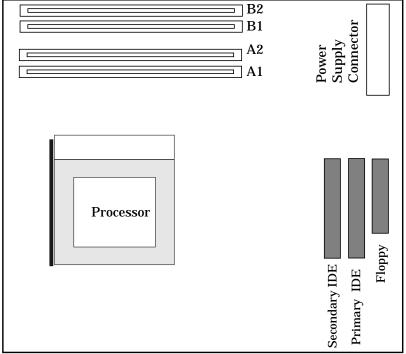
If only two RDRAM modules are installed, use the sockets marked A1 and B1. The other two sockets (A2 and B2) must contain continuity modules.
